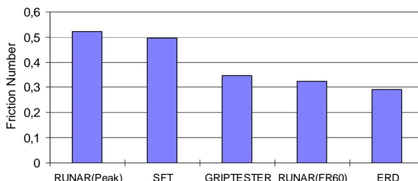
Figure 10 - Correlation between friction devices on snow- and ice-covered runways from North Bay, 1996.
