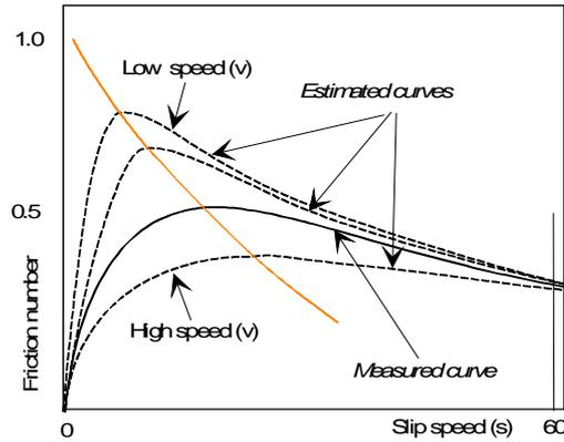
Figure 14 - A sample FrictionPrint for wet pavement.
