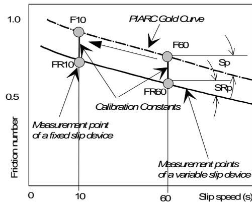
Figure 17 - Calibration of a fixed slip device.
