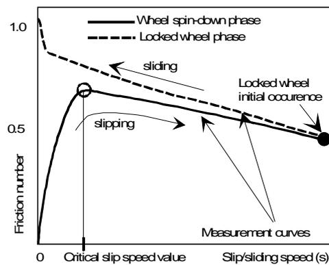
Figure 2 - Friction number graph for a locking brake.
