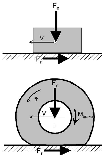
Figure 1 - Free body diagrams of a sliding block and a braked wheel.
