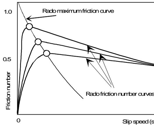
The Norsemeter friction measuring devices utilize what is called a variable slip measuring technique.
