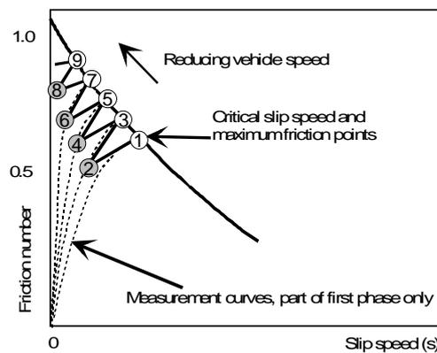
Figure 4 - Friction number graph for anti-lock brake system.
